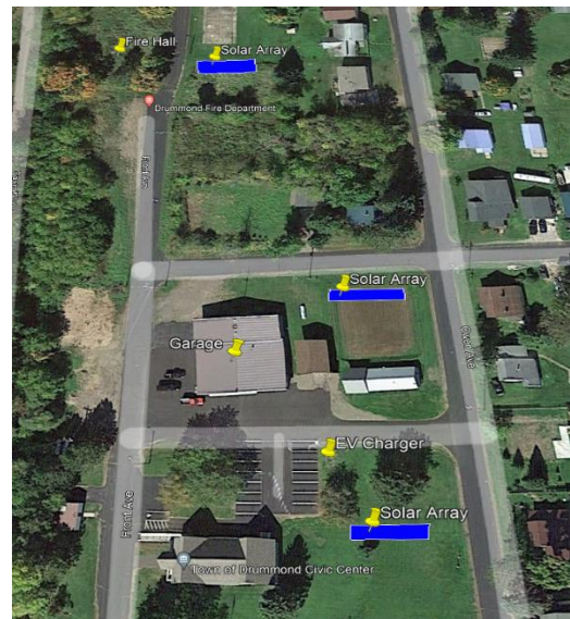
Figure 7. Town of Drummond 5% microgrid layout
